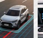
The system identifies the marker lines of the lane where the car is running through the front-view camera, and calculates the car's location relative to the lane. When the driver is unaware of diverging from the lane, the system will give an alert to remind the driver of
